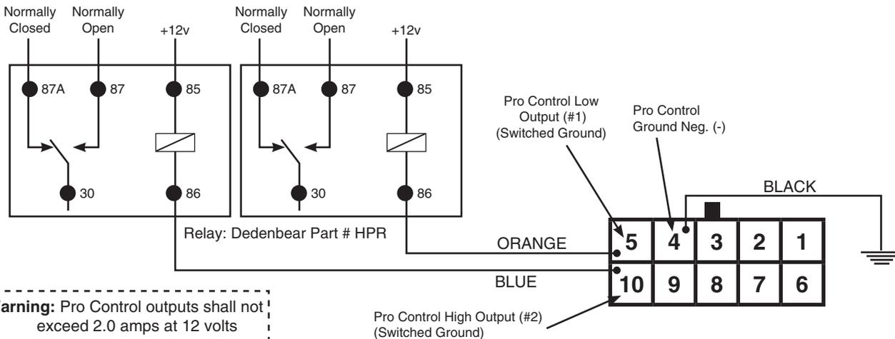
**Warning:** Pro Control outputs shall not exceed 2.0 amps at 12 volts
